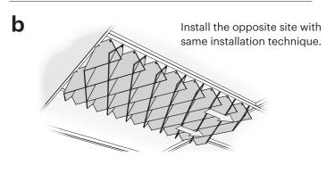
On adjacent side, further expand the Clario baffle so that the slots are captured by the T-grid.
