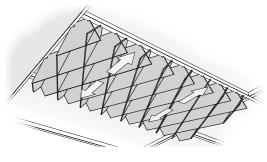
Repeat on the last side with same installation technique. Orient additional baffles in the same direction.
