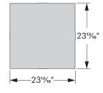
**e** To trim Tetria Tiles, measure opening dimension from "on center" or spline dimension.
