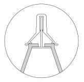
After installing two adjacent Tetria Tiles, reach up above the grid through an adjoining open space (where a tile has not been placed yet) and place the clip on the cross tee to push the Tetria Tile down in place.
