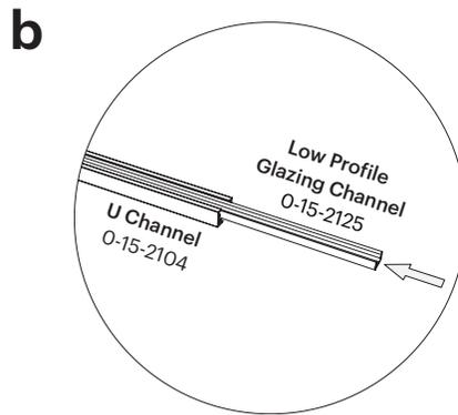
Insert Glazing Channel (0-15-2125) into U Channel (0-15-2104).
